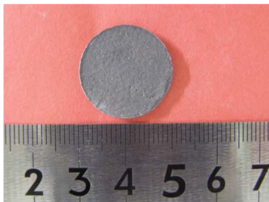
Fig. 6 Outside appearance of the bulk prepared by the HHP treatment of titanate nanotubes with a Pt salt under 40 MPa at 423 K for 2 h and a subsequent heat-treatment at 573 K in H_2
